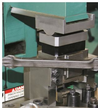
Pickets-flatten end and shear corners in one step.
