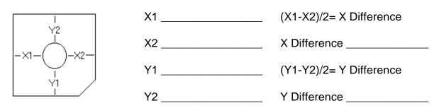
While determining the difference value to input, keep the following in mind: When adjusting the X on ALL models, a positive (+) value will make X1 smaller When adjusting the Y on ALL models, a positive (+) value will make Y1 smaller
